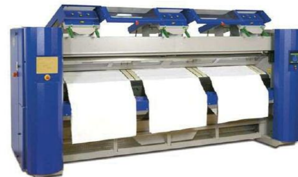
CONVEYED BY SUCTION: Raising the load stations reveals a powerful suction conveyor that can be used to feed small pieces or irregularly shaped linen, such as a round table cloth, that does not fit conveniently into the loading clamps
